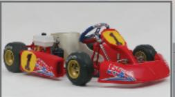
The B25 comes standard with the Birel MTS\* accessory package and turn-key COMER C-50 engine package. The kart also features Bridgestone YJL tires and Freeline bodywork.
